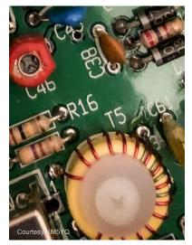
The third phase of the K2 build is to install the remaining band pass filter, low pass filter and the transmitter components. Another decent size group of resistors and a large group of capacitors were the first big steps. Somewhat tedious, but these are the steps where it is important to take your time, and several breaks. After this, the build went much quicker as I had already pre-wound the remaining toroids.
