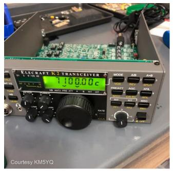
A while back, I built an Elecraft KX3. As with a K3, it was mostly a screw-together job with pre-soldered boards. My goal with the K2 was to have a full-featured HF rig that I totally built myself before kits like this are no longer available.
