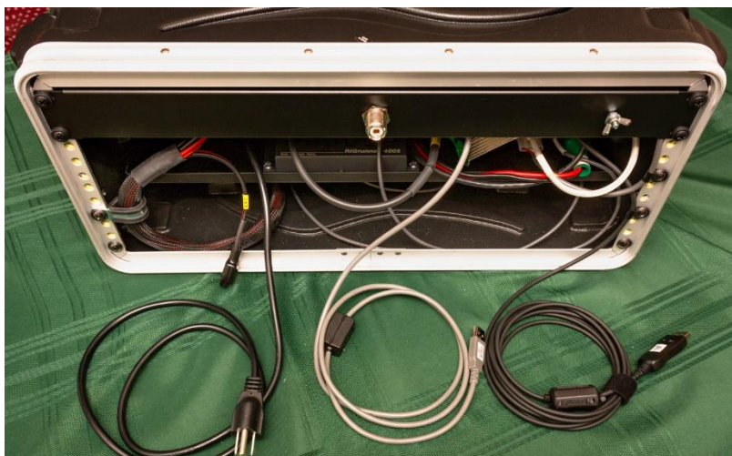
HF Kit rear view showing antenna connector brought out to the rear panel because it's not accessible otherwise. Cables L to R: AC power; SignalLink USB; Icom CI-V USB
